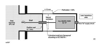
et teatatuction without a fior actualistic and the anti-Figure 2 - Example of a separation element with a cylindrical shaft joint and natural ventilation
